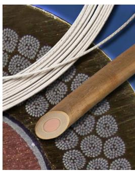
Supercon High Field Superconducting Wire provides a 16-18 K transition temperature and a high critical magnetic field for applications >10 Tesla. Available as stabilized or non-stabilized conductors, it can be supplied as bare or braided fiberglass insulted wire or cable.
